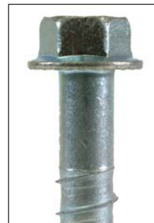
The Titen HD 3/4 x 6 and 3/4 x 7 have a 1" section under the head that is unthreaded to allow installation into tilt-up wall braces.
